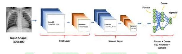
Pneumonia Detection using Convolutional Neural Network (CNN)
